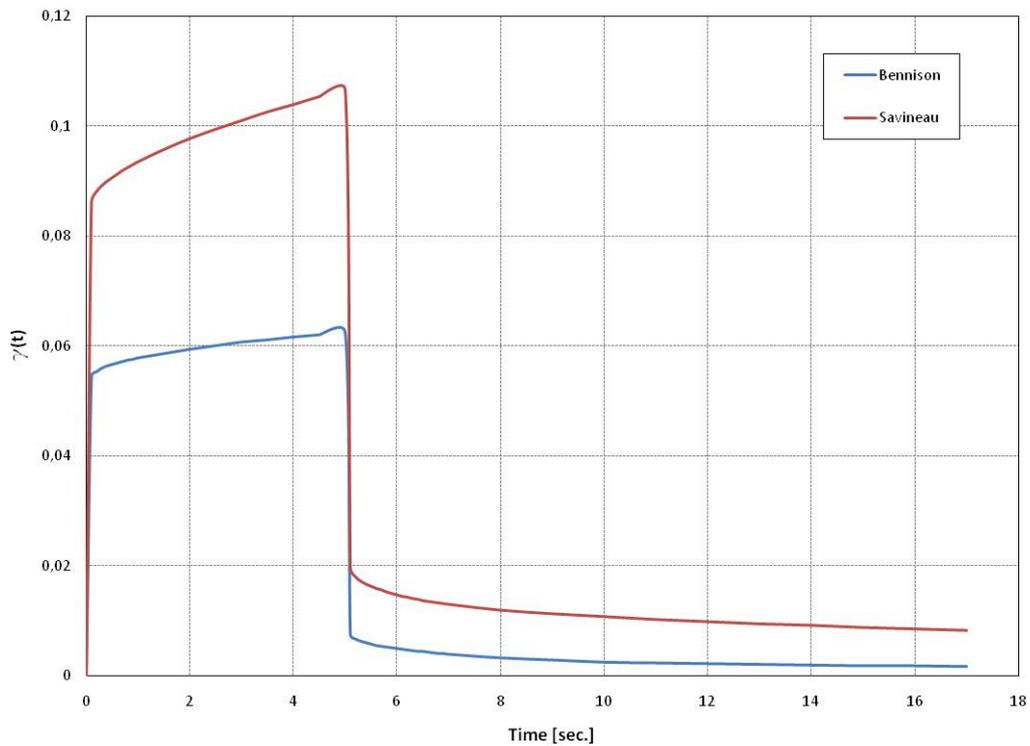
*Fig. 6 – Shear deformation  $\gamma(t)$  vs. time in numerical creep analysis*
