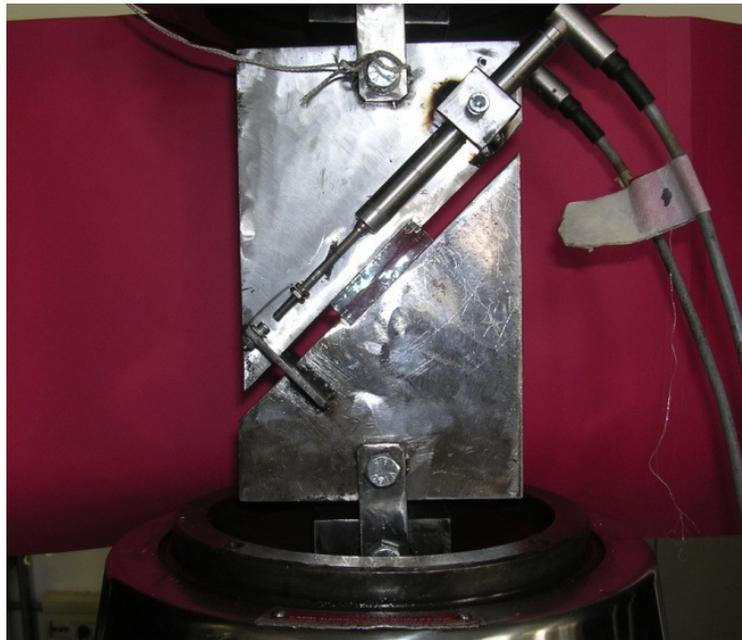
Fig. 2- CST test device
