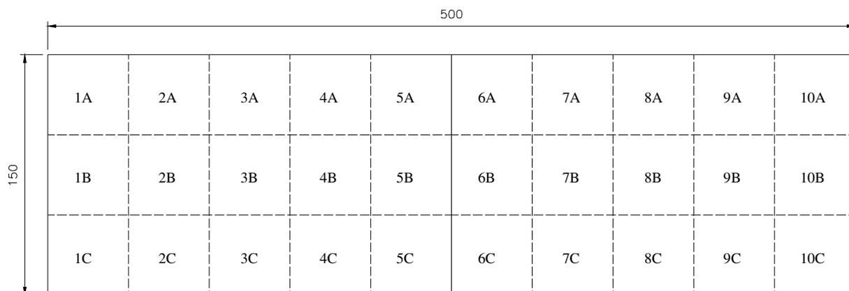
Fig. 1- Labelling and location of the specimens over the original LSG pane.
